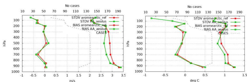
Fig.4: bias and standard deviation for wind speed (left) and temperature (right) for the reference experiment (red) and the experiment assimilating all Aeolus observations (green).
