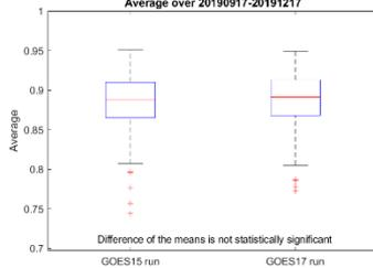
Box/whisker plots show some differences even though the difference in means is not statistically significant. The whiskers enclose approx.  $\pm 2.7\sigma$ , with the whisker plotted at the ob closest to and inside that limit. Note the difference in the lower whisker placement for GOES-17.
