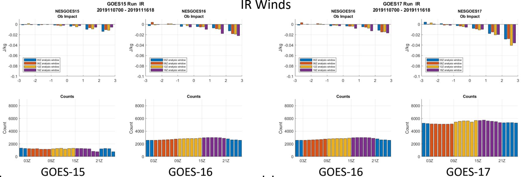
NESGOES-17 IR AMVs provide beneficial impact even during the periods with high focal plane temperatures and despite the reduced counts.
