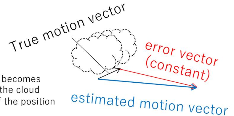
As the observation time interval becomes smaller, the moving distance of the cloud becomes smaller, so the error of the position vector increases relatively.
