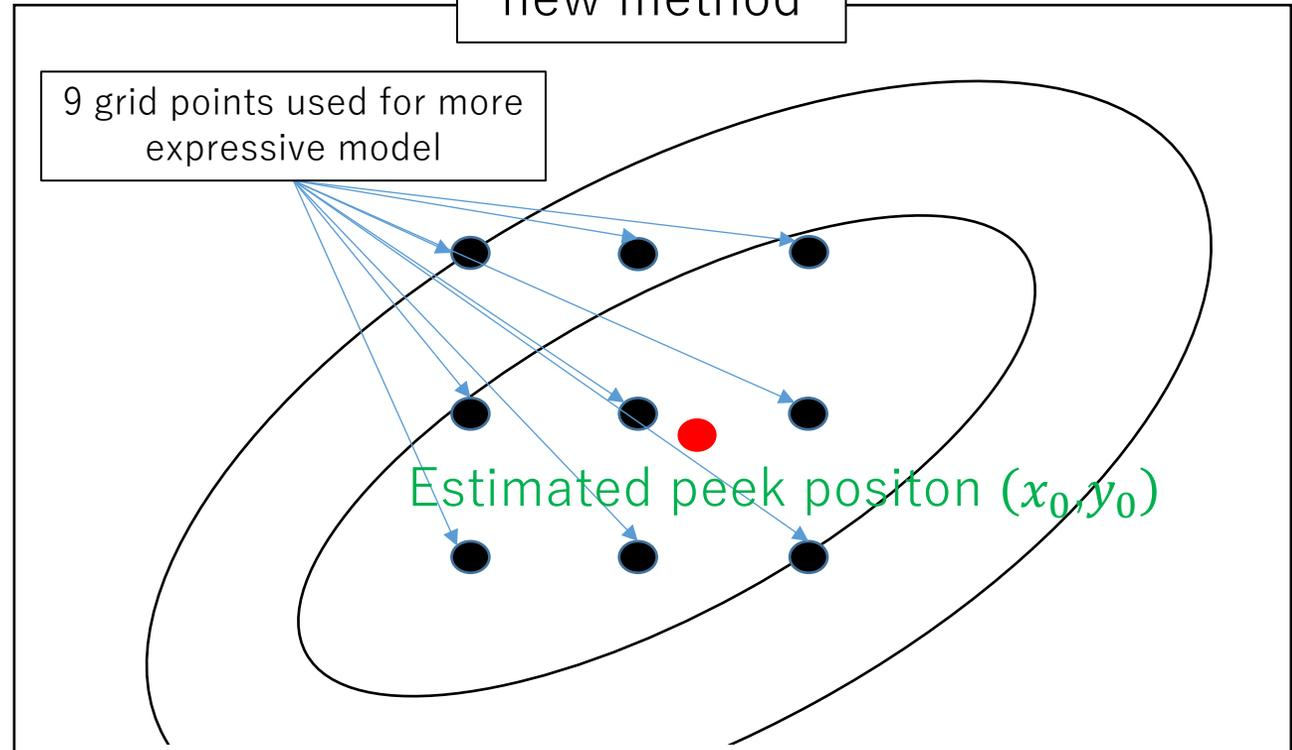
$$C(x, y) = a(x - x_0)^2 + b(y - y_0)^2 + c + d(x - x_0)(y - y_0)$$
