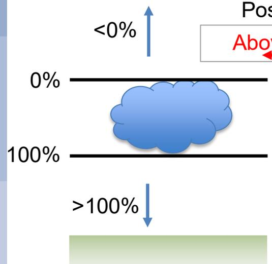
More sensitivity to height assignment errors in regions of greater wind shear above cloud
