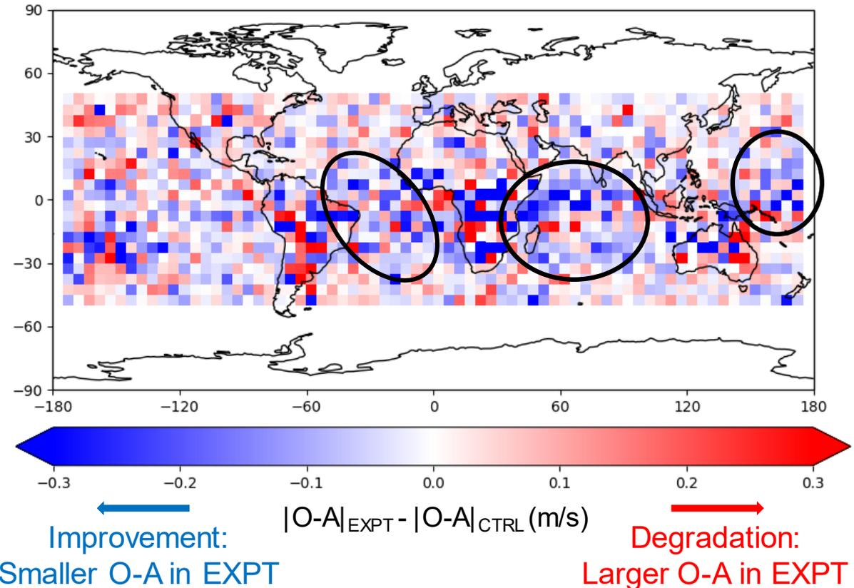
Reduction in O-A to support changes due to AMV processing
