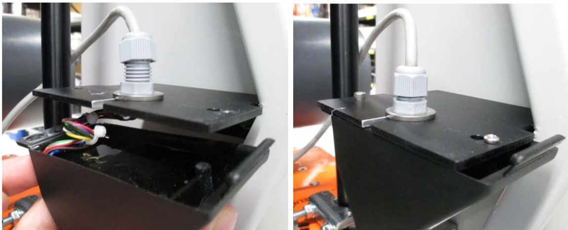
Figure F- 18. Rain sensor re-installed
