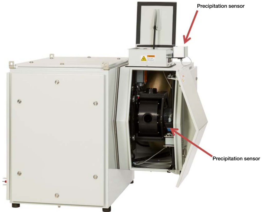
Figure F- 5. Precipitation sensor location
