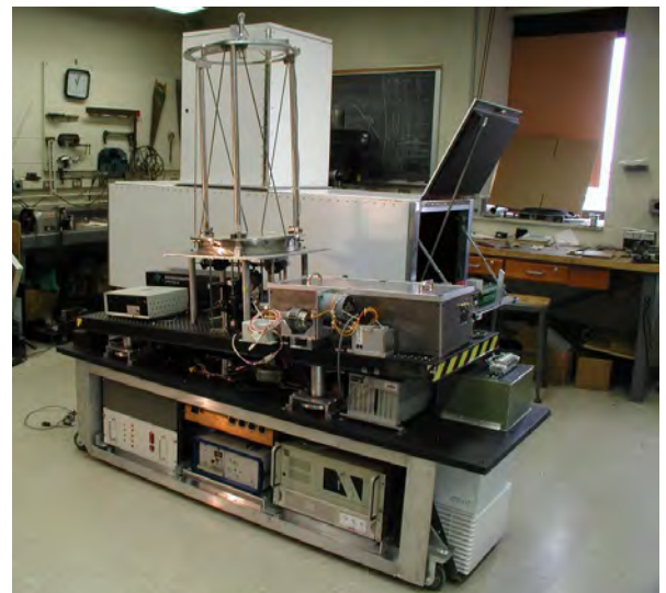
The LIDAR with the environmental housing removed.
