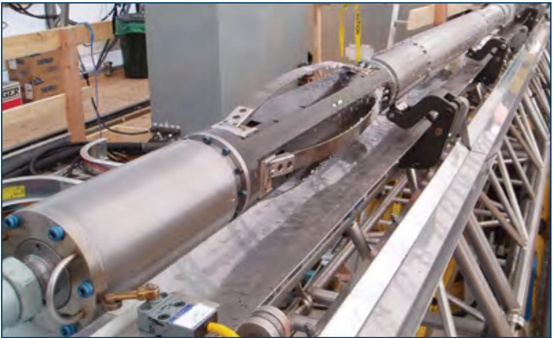
An ICDS team tested the DISC drill in Greenland during summer 2006. In the image on the left, an ICDS technician removes the DISC drill's first core from the core barrel. On the right, the drill sonde sits on the tower. When upright, the tower supports the sonde as it descends into the hole and later returns to the surface. The map shows the WAIS Divide site.
