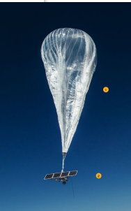
Loon balloon with payload platform Photo Credit: Loon - https://loon.com/
